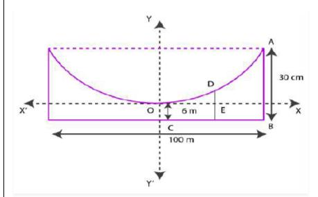
Here, AB and OC are the longest and the shortest wires, respectively, attached to the cable.
