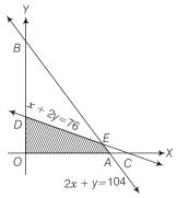
**Sol.** As clear from the graph, corner points are *O*, *A*, *E* and *D* with coordinates (0, 0), (52, 0), (144, 16) and (0, 38), respectively. Also, given region is bounded.
