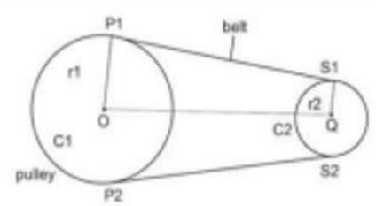
Given is the diagram of a pair of pulleys. C1 and C2 are two pulleys attached with a belt. P1 and P2 are position of contact, where the belt meets C1. S1 and S2 are point of contact, where belt meets C2. O and Q are the centres of C1 and C2, respectively
