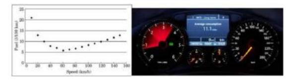
The relation between fuel consumption F(l/100km) and speed V (km/h) under some constraints is given as  $F = \frac{V^2}{500} - \frac{V}{4} + 14$ .
